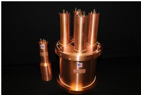
Figure 4. NaI(Tl) 9" x 9" Annulus and Plug Detector.
