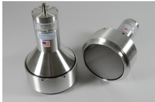
Figure 2. Special F.I.D.L.E.R. Thin Integral Detectors with beryllium energy entrance windows.
