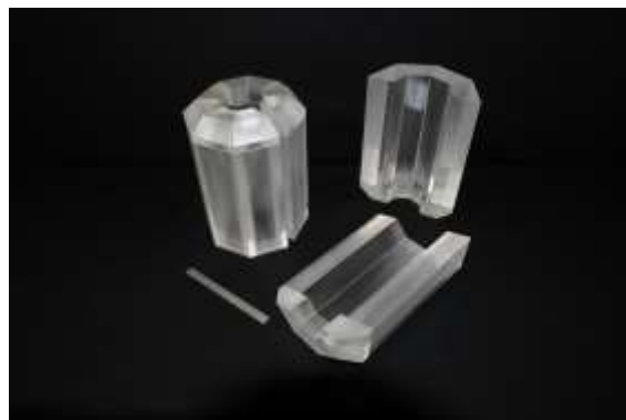
Figure 2. Segmented BGO Crystal Blanks for the Detectors shown in Figure 1.
