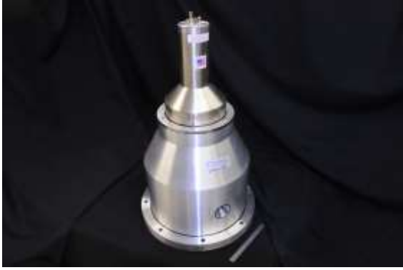
Figure 4. Special large Compton Suppressor with Side and End Well for INEL
