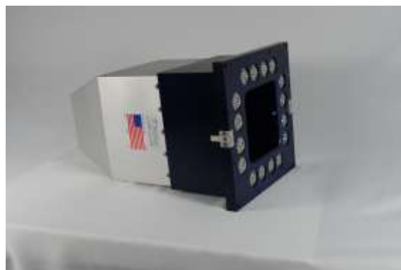
Figure 3. BGO Compton Suppressor for the Clover System at LLNL.
