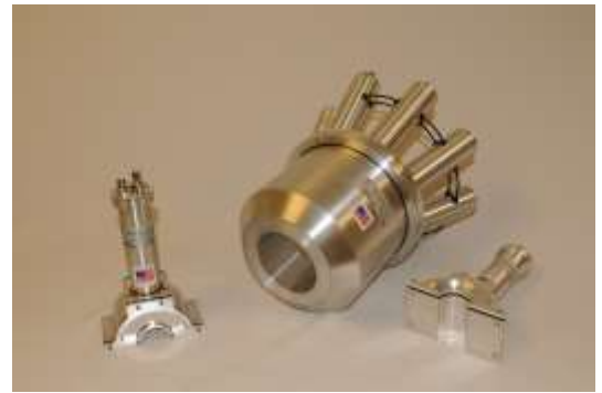
Figure 7. Another BGO Annulus Design Shown with "Backcatcher" Detectors
