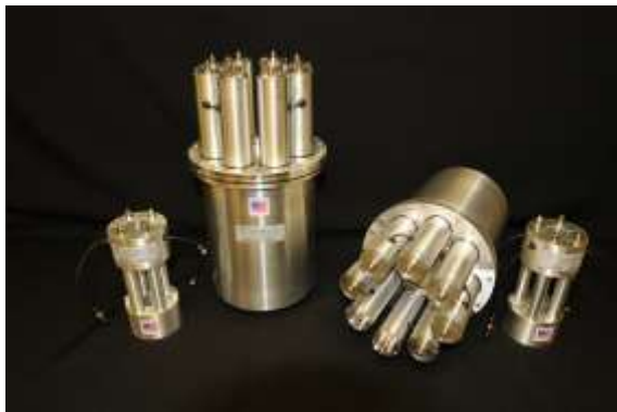
Figure 1. BGO Annulus and “Backcatcher” Detectors.
