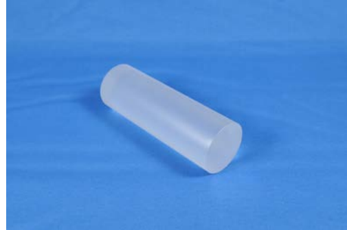
Figure 1. BGO crystal blank. (ASI photo)
