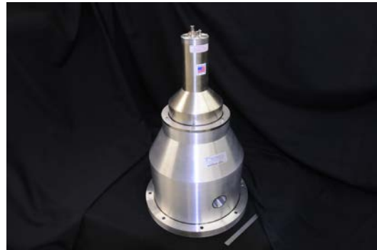
Figure 8. ASI Very Large BGO Annular Detector showing complete assembly.
