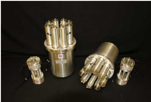
Figure 6. ASI BGO Annular Detector BGO completed assembly.
