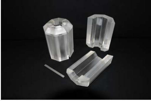
Figure 5. ASI BGO Annular Detector BGO segmented crystal blanks shown.
