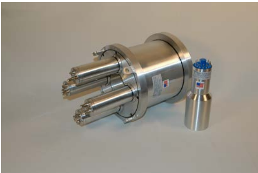
Figure 1. NaI(Tl) 9" x 9" Axial Through Well Annulus with Plug Detector.
